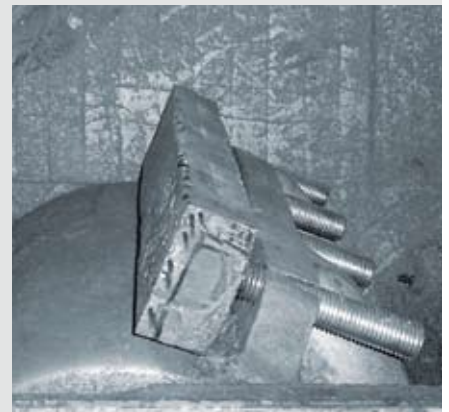
Glass recycling; impact crusher for crushing of ceramics
